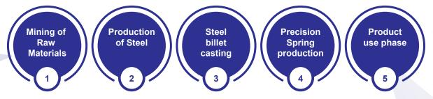
MyTech is involved in stage 4 of the industry where the precision spring production process entails, with some variations based on the type of spring being made, a process of winding, heat treating, grinding, coating and finishing.
